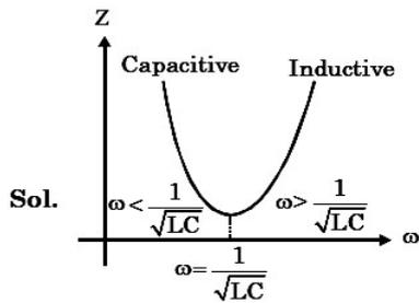
Sol. The circuit will have inductive nature if  $\omega > \frac{1}{\sqrt{LC}}$  ( $\omega L > \frac{1}{\omega C}$ ) Hence A is false. Also if circuit has inductive nature the current will lag behind voltage. Hence D is also false.
